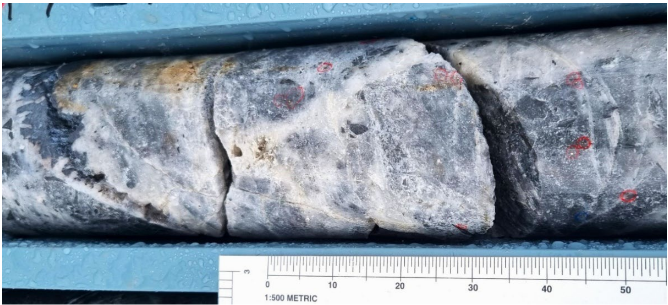
Figure 6 Drill core from BKC018 at 412.6m depth interpreted to be in the Little Reef mineralised zone. Assays for the interval 412.6 to 413.36m returned 104.29 g/t Au and 0.77% Sb. The red-circled points on the core are visible gold grains.
