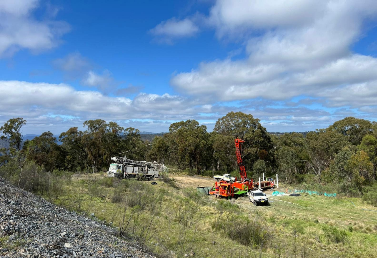
Figure 1 Diamond rig (red) drilling and RC rig (white) moving onto pre-collar No 2 at Garibaldi
