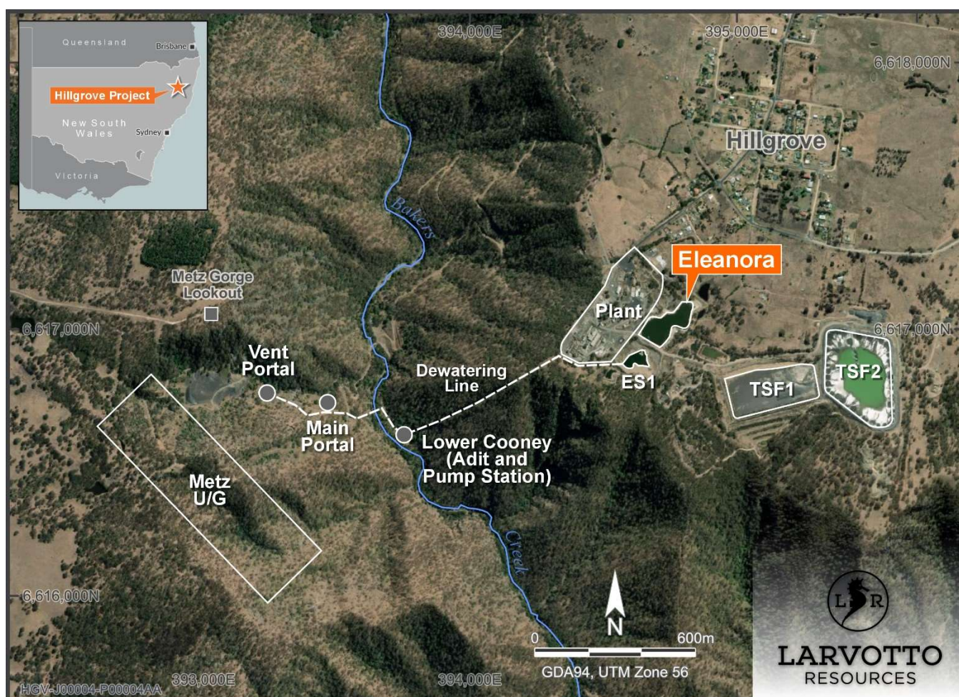
Figure 11 The main water management infrastructure at Hillgrove Mine
